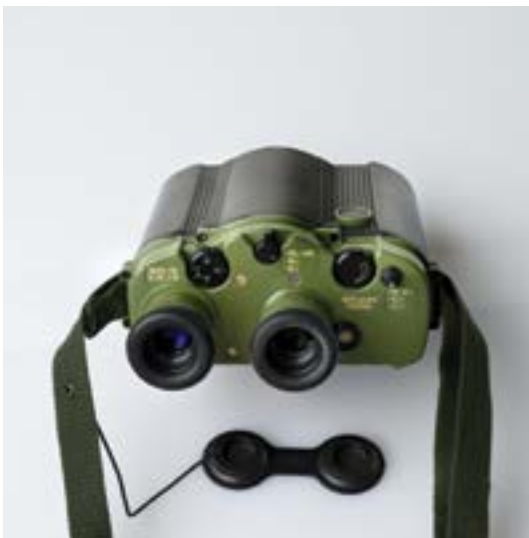
Janja Lap, miniature laser rangefinder/distance meter RLD-2 (product photograph), 1981, h: 9 cm, w: 22.5 cm, l: 18 cm, Iskra Elektrooptika, photo: Miran Kambič. Private property.
