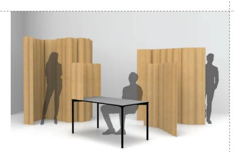
**Figure 3:** The module of 760 x 650 mm size is the desktop version of the soundproofing partition; the 1520 x 650 mm size is intended for spaces where people tend to be sitting down; the large 1900 x 860 mm module is designed to serve as a partition in open spaces, like fairgrounds. It is used to create a quiet environment inside noise-saturated halls or large rooms. The 2280 x 1025 mm model is intended for completely partitioning spaces and creating entirely new rooms.
